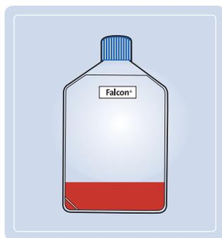
7. After mixing or adding cell suspension, place the Falcon® Multi-Flask vertically on a flat work surface to equalize liquid volume among all the layers.
