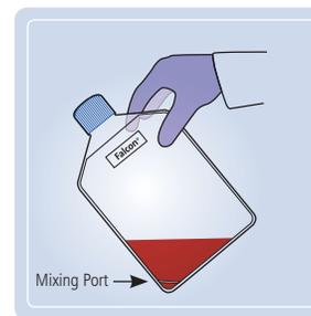
4. Mix position: Hold the Falcon Multi-Flask upright with the logo facing you and tilt counter-clockwise to a 45° angle.
