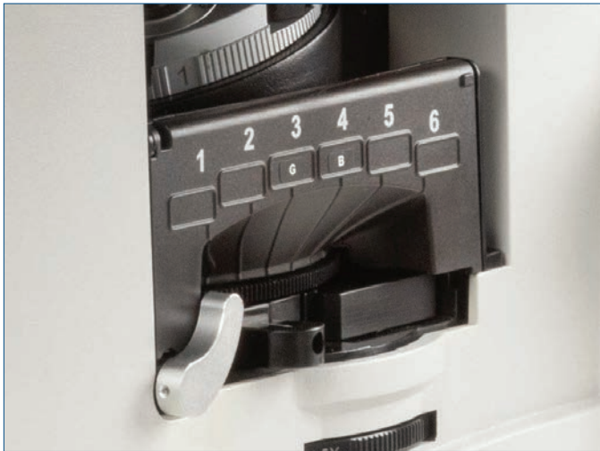
6-Position fluorescence filter set wheel
